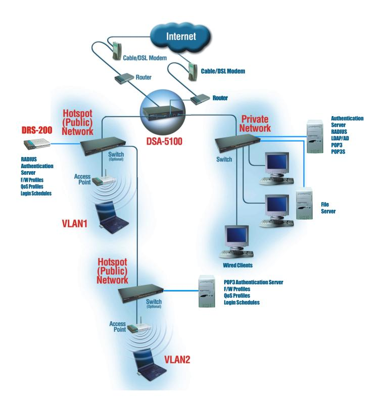
To cost-effectively double your Internet bandwidth, you can (1) connect both WAN ports of your AirSpot Gateway to two separate lower rate/lower charge broadband lines, then (2) allocate your users/servers' traffic to different WAN ports to create an even load balance.
